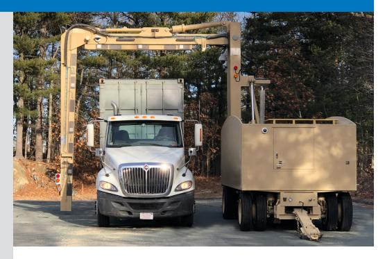
The Rapiscan Eagle® T25 is a trailer-mounted, drive-through inspection system with material discrimination for efficient screening of cargo for threats and contraband. The fully self-contained unit can be easily towed and rapidly deployed. The system offers portal mode operation with automatic cab exclusion or CabScan® mode to image the entire vehicle. Vehicles are scanned as they drive through the tunnel at 3–8 km/hr (2–5 mph).
