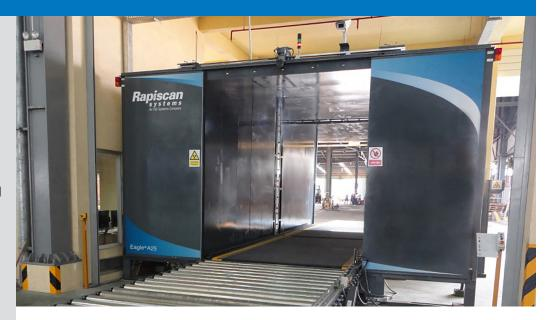
The Rapiscan Eagle® A25 is an advanced X-ray system for scanning pallets and unit load devices (ULDs) to produce high-quality images with three-color material discrimination. Cargo moves through the inspection tunnel on a conveyor system with entrance and exit conveyors that facilitate loading and unloading of containers and pallets. The Eagle A25 system has integral shielding, which reduces the radiation exclusion zone to the boundary of the system.
