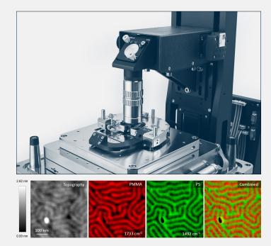
"Integrating Block's QCLs into our atomic force microscope (AFM) has enabled us to acquire both topography, IR spectra and spectral mapping with ~ 5 nm spatial resolution, about 1000X better than the resolution of the FTIR microscopes."
