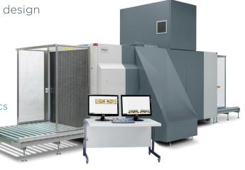
The Rapiscan 632DV is an advanced cargo and large parcel system designed for inspection of pallet and break bulk cargo screening. The Rapiscan 632DV tunnel opening of 1,500 mm x 1650 mm, automatic detection of explosives, dual view technology, and superior image quality allows high throughput of screened objects.
